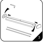
3. Peel off the cover. You'll get a screwdriver in the cover and two telescopig poles in the base unit.
