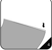
4. Paste aluminium bars one by one upon the upper and down edges of the graphic.
