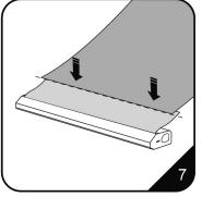
7. Peel off the adhesive cover along the edge of the base's leader roll, and attach the bottom of the banner tape along the inside of the edge. (front facing up).
