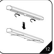
12. Two revolving feet to strenghten stability.
