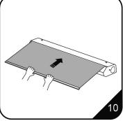
10. Carefully allow the graphic to recoil into the base unit (it may be useful to have an assistant hold the base steady).
