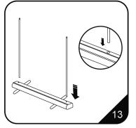
13. The bottom of the assembled pole slides into the round socket in the base unit.
