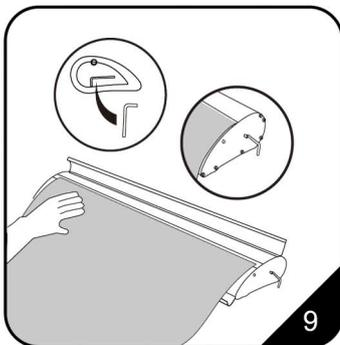
9. Activate the spring tension by removing the Allen Key. Pull the Allen Key while holding on the the attached graphic. Save the key in the side cover.
