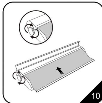
10. Carefully circumgyrate the tension circle, make the graphic go into the base unit.
