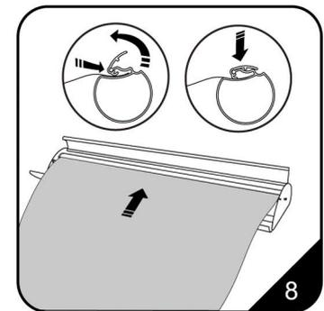
8. Open the roller's lid, slide the bottom edge of the graphic under the lid. Close the roller's lip to secure the graphic.
