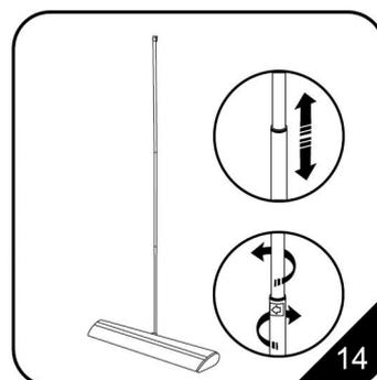
14. Draw out the upper of the telescopic pole to adjust the height to suitable level, then circumgyrate to firm it.
